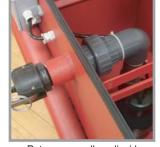
Return pump allows liquid return at 38 gallons/minute.
